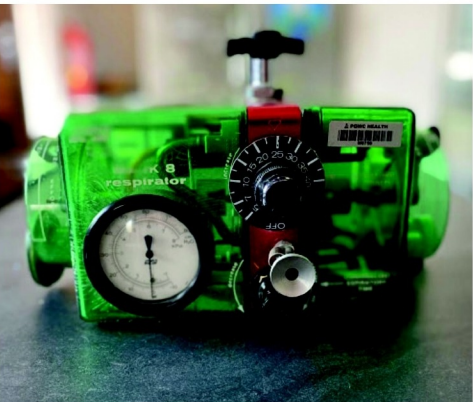
An existing mechanical respirator being reverse-engineered to be used as an emergency ventilator.
